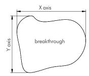
With the dimension of the smallest "light width", it should be checked whether a pipe sleeve has space in the breakthrough.
