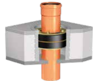
Variant: Curaflex® 3000 and Curaflex® C as bottom feed-through
