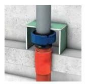
$Curaflam^{\text{\tiny{\it B}}}\; Konfix^{\text{\tiny{\it Pro}}}\; penetration\; sealing$ (including further ducts if applicable) must be clad behind a shell made of fire-proof cement or plaster-composite panels measuring at least 9.5 mm thick (e.g. drywall) or clad in solid materials measuring at least 50 mm thick.
