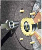
Punching out holes with the punch tool
