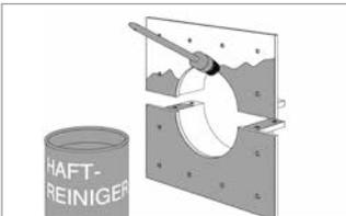
Pretreatment of the steel pipe sleeve with Sika Adhesion Cleaner-1. Apply to the back of the steel plate (against the sleeve) and to the dividing plates using a brush or cloth.
